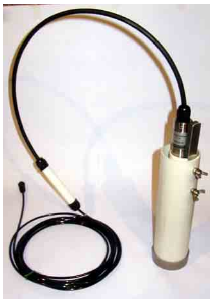
The water depth sensor is put inside the stilling well.
