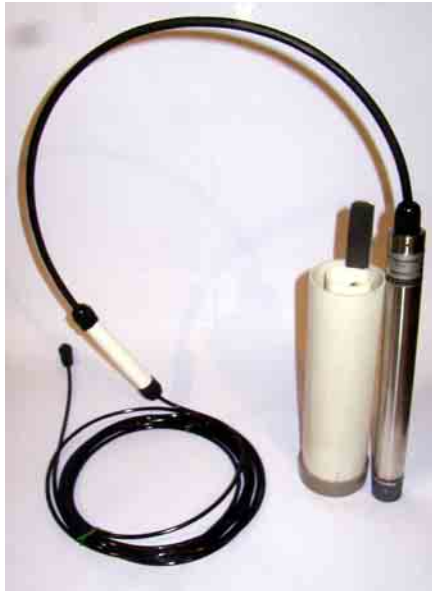
Water depth sensor and stilling well.
