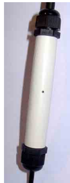
A small air hole in the water depth sensor cable provides atmospheric pressure to the sensor.
