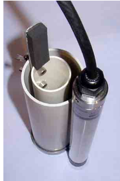
Water depth sensor and stilling well detail.
